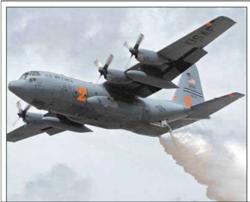
Tech. Sgt. Rick Sforza / U.S. Air Force A C-130 Hercules, equipped with a Military Airborne Fire Fighting System, drops water during annual MAFFS training in New Mexico. Six of the C-130s have been dispatched to help battle wildfires in California.
